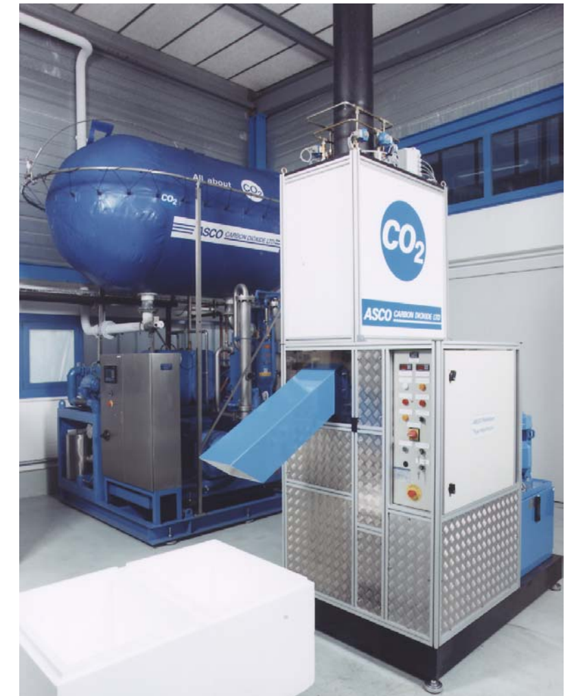
Pelletizer P600 connected to a Revert Recovery System
